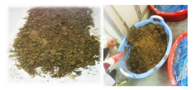
Fig. 3. Mixing the fuel oil with the soil in the laboratory of University of Baghdad.
