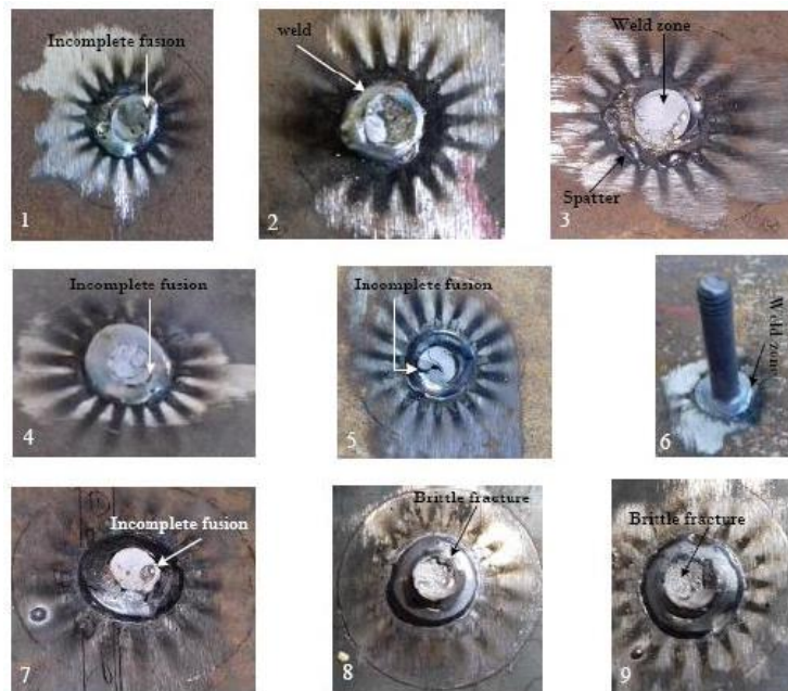
Fig. 9. The fractured specimens by torsional test.
