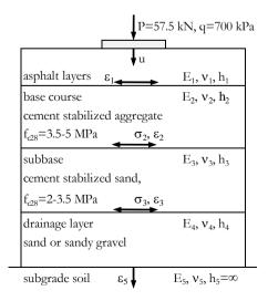
Fig. 1. Model of pavement structure (first construction stage).
