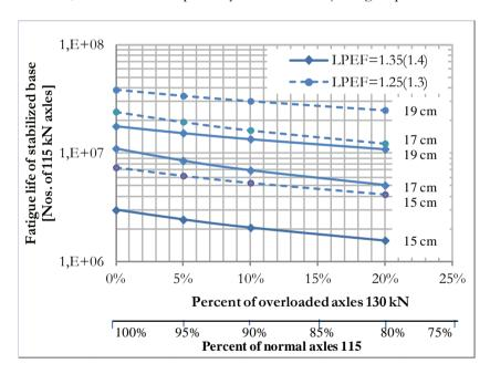
Fig. 7. Total number of axle loads to fatigue cracking of stabilized base in relation to percentage of overloaded axles, thicknesses of asphalt layers and LPEF (different temperatures for four seasons).
