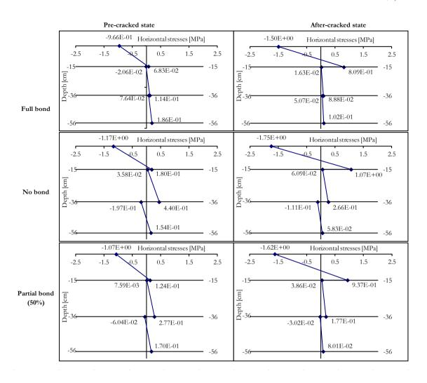
Fig. 2. Horizontal stresses in pavement layers ("-" compression, "+" tension) for pre-cracked and after cracked state in relation to bond between cement stabilized layers.
