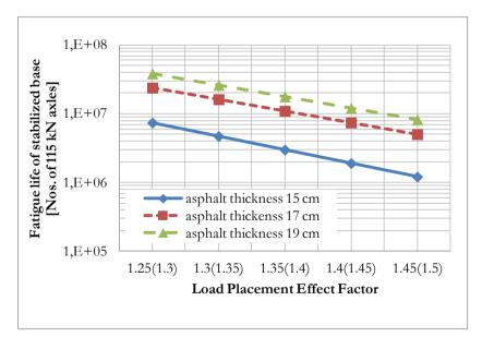
Fig. 4. Fatigue life of cement stabilized base in relation to LPEF and thicknesses of asphalt layers (average annual equivalent temperature +12°C).
