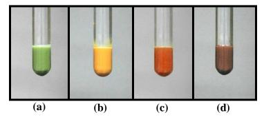
Fig. 2. The change of suspension color appeared during the reaction between copper salt and polyol at the reaction temperature of 140 °C and molar ratio of NaOH:Cu(NO<sub>3</sub>)<sub>2</sub> = 2:1 at different reaction period (a) 20, (b) 30, (c) 120, and (d) 240 minutes after heating the solution.
