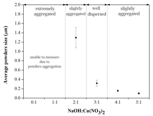
Fig. 5. Average powder sizes as a function of the concentration of sodium hydroxide.
