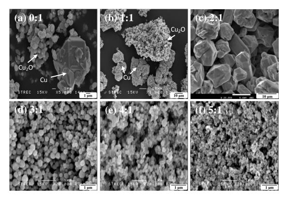
Fig. 4. The morphology of the powders obtained from different molar ratio of NaOH:Cu(NO<sub>3</sub>)<sub>2</sub> at the reaction temperature of 140 °C : (a) 0:1, (b) 1:1, (c) 2:1, (d) 3:1, (e) 4:1 and (f) 5:1.
