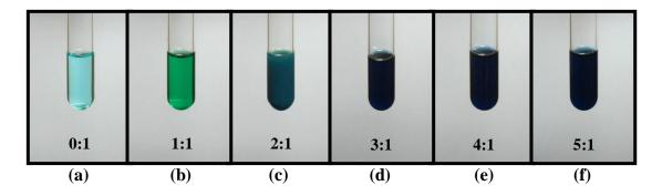
Fig. 1. Color change of solution after mixing NaOH in various molar ratios of NaOH:Cu(NO<sub>3</sub>)<sub>2</sub>: (a) No NaOH addition, (b) 1:1, (c) 2:1, (d) 3:1, (e) 4:1, and (f) 5:1.
