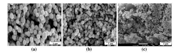
Fig. 6. The morphology of the copper powders prepared using the constant molar ratio of  $NaOH:Cu(NO_3)_2 = 3:1$  at various reaction temperatures (a) 120 °C, (b) 140 °C, and (c) 160 °C.
