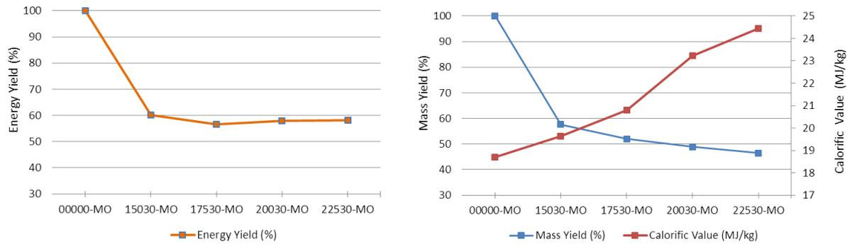
Fig 12. Effect of temperature on energy yield of mixed organic waste (left) and comparison between mass yield and calorific value of raw and products from mixed organic waste (right).
