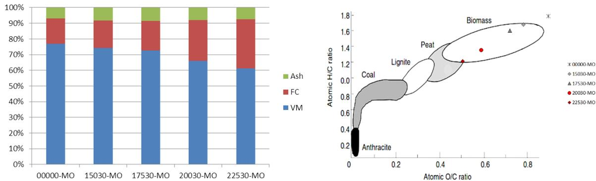
Fig. 11. Physical properties (left) and chemical properties (right) of raw and products from mixed organic waste.
