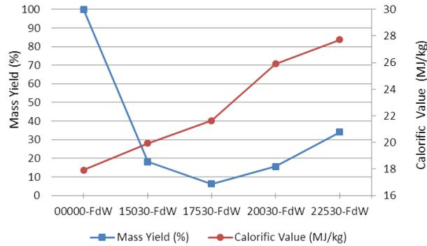
Fig 10. Effect of temperature on mass yield and calorific value of food waste.
