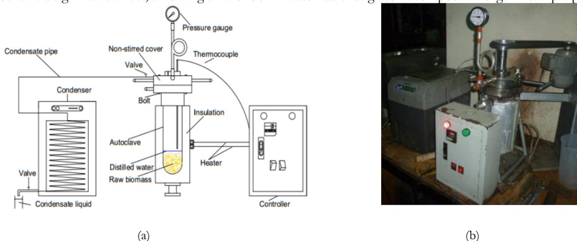
Fig. 1. Schematic (a) and installation (b) of lab scale reactor.
