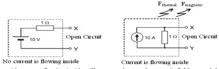
Fig. 2. The box with current flowing inside will generate heat and magnetic field around the conductor.
