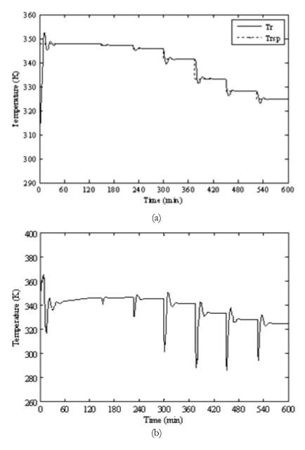
Fig. 9. The temperature control using PID control under the nominal case: (a) the control variable  $(T_r)$  and (b) the manipulated variable  $(T_{isp})$ .
