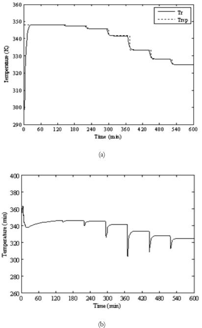
Fig. 7. The temperature control using NNMPC under the nominal case: (a) the control variable ( $T_r$ ) and (b) the manipulated variable ( $T_{isp}$ ).
