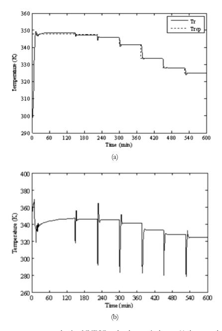
Fig. 8. The temperature control using NNDIC under the nominal case: (a) the control variable ( $T_r$ ) and (b) the manipulated variable ( $T_{jsp}$ ).
