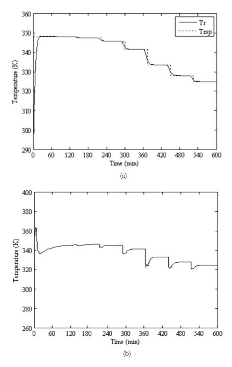
Fig. 10. The temperature control using NNMPC under the parameter mismatch case (-30% U): (a) the control variable ( $\Gamma_r$ ) and (b) the manipulated variable ( $\Gamma_{jsp}$ ).
