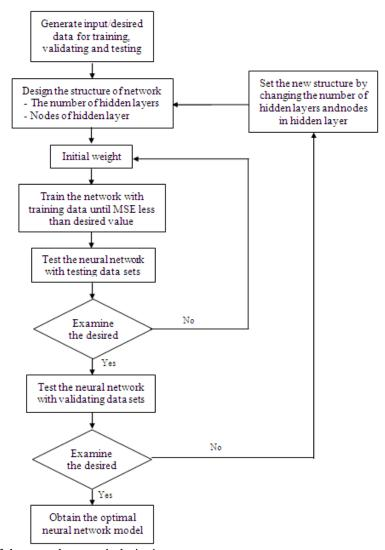
Fig. 2. Procedures of the neural network designing.
