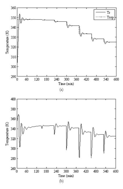
Fig. 11. The temperature control using PID control under the parameter mismatch case (-30% U): (a) the control variable ( $T_r$ ) and (b) the manipulated variable ( $T_{jsp}$ ).
