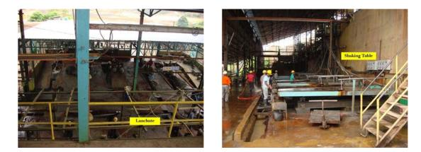
Fig. 4. Apperance of Lanchute and Shaking Table.
