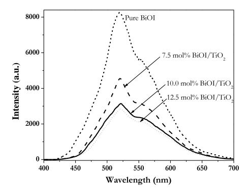
Fig. 6. Photoluminescence (PL) spectra of pure BiOI, 7.5 mol% BiOI/TiO<sub>2</sub>; 10.0 mol% BiOI/TiO<sub>2</sub> and 12.5 mol% BiOI/TiO<sub>2</sub>, repectively.
