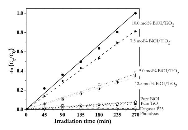
Fig. 7. Pseudo-first order degradation rate of photocatalytic degradation of phenol over the catalysts.
