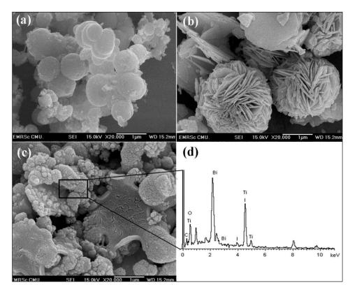
Fig. 2. FE-SEM images of (a) Pure TiO<sub>2</sub>; (b) Pure BiOI; (c) 10.0 mol% BiOI/TiO<sub>2</sub> composite and (d) the EDX spectrum of (c).
