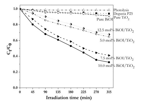
Fig. 5. Phenol photodegradation efficiencies over synthesized catalysts.
