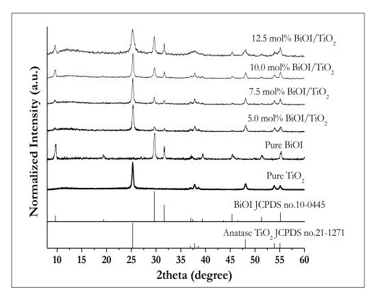
Fig. 1. XRD patterns of pure TiO<sub>2</sub>, pure BiOI and BiOI/TiO<sub>2</sub> nanocomposites.
