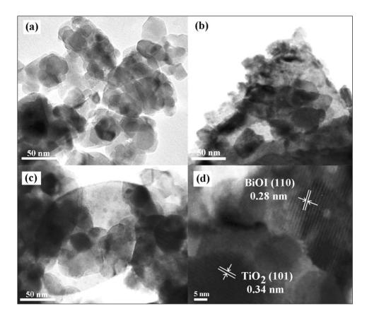
Fig. 3. TEM micrographs of (a) pure TiO<sub>2</sub>, (b) pure BiOI and (c,d) 10.0 mol% BiOI/TiO<sub>2</sub> nanocomposite.
