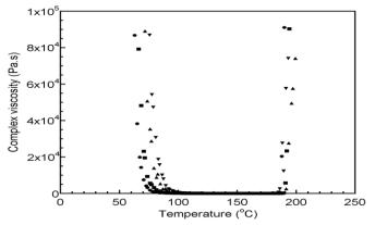
Fig. 4. Processing window of benzoxazine molding compound with different nano-SiO<sub>2</sub> contents: (•) 1wt%, (•) 3wt%, (•) 5wt%, (•) 7wt%, (•) 10wt%.
