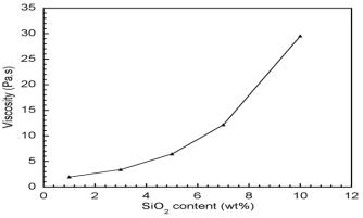
Fig. 3. Relation between nano-SiO<sub>2</sub> content and viscosity of benzoxazine molding compound
