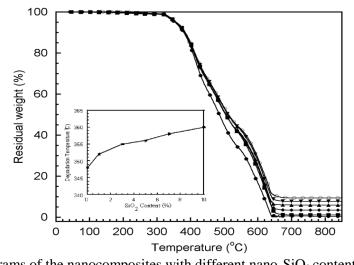
Fig. 5. TGA thermograms of the nanocomposites with different nano-SiO<sub>2</sub> contents: (•) neat polybenzoxazine, (•) 1wt%, (•) 3wt%, ( $\blacktriangle$ ) 5wt%, ( $\blacktriangledown$ ) 7wt%, ( $\circ$ ) 10wt%. Inset of Fig. 5. Degradation temperature at 5% weight loss of nano-SiO<sub>2</sub> filled polybenzoxazine with various nano-SiO<sub>2</sub> contents.
