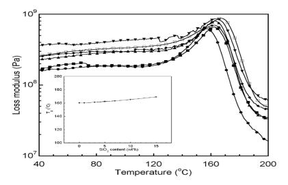
Fig. 9. DMA thermograms of loss modulus with various nano-SiO<sub>2</sub> contents: (•) neat polybenzoxazine, (•) 1wt%, (•) 3wt%, (•) 5wt%, (•) 7wt%, (•) 10wt%.
