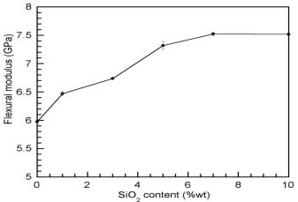
Fig. 6. Relation between nano-SiO<sub>2</sub> content and flexural modulus of nanocomposites.
