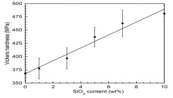
Fig. 10. Relation between nanofiller content and micro Vickers hardness of nano-SiO<sub>2</sub> filled polybenzoxazine.
