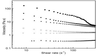
Fig. 2. Viscosity of benzoxazine molding compound with different nano-SiO<sub>2</sub> contents at 120 °C: ( $\blacktriangle$ ) benzoxazine monomer, ( $\circ$ ) 1wt%, ( $\square$ ) 3wt%, ( $\blacklozenge$ ) 5wt%, ( $\blacksquare$ ) 7wt%, ( $\blacksquare$ ) 10wt%.
