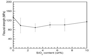
Fig. 7. Relation between nano-SiO<sub>2</sub> content and flexural strength of nanocomposites.
