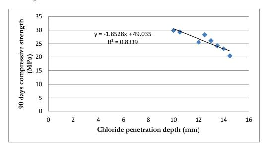
Fig. 3. Chloride penetration depth vs compressive strength at 90 days.
