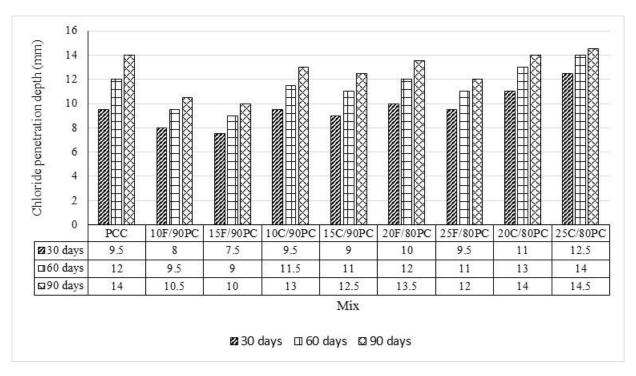
Fig. 2. Chloride penetration depth of full immersion in 3% NaCl solution.
