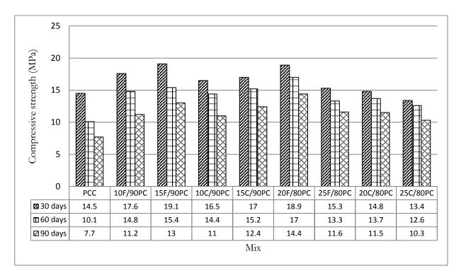
Fig. 4. Compressive strength of cube samples in 5% sulphuric acid.
