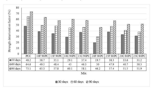
Fig. 5. Strength deterioration factor of cube samples.
