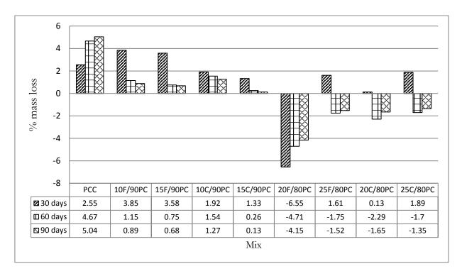
Fig. 6. Percentage mass loss of cube samples in sulphuric acid.
