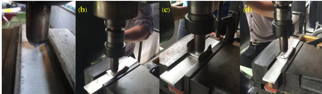
Fig. 2. The friction stir spot welding process.
