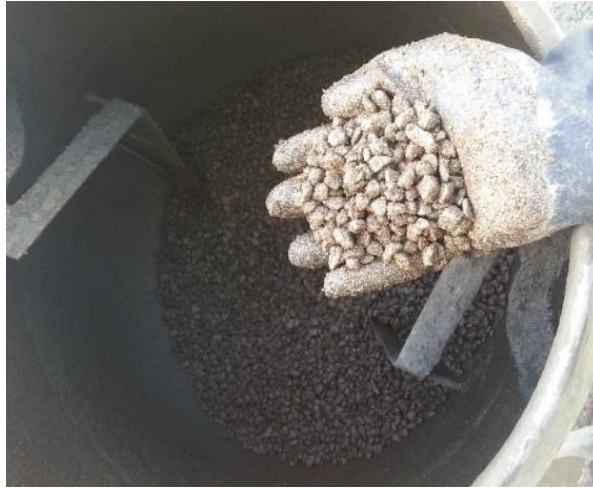
Fig. 8. Covering of coarse aggregates by vermiculite.
