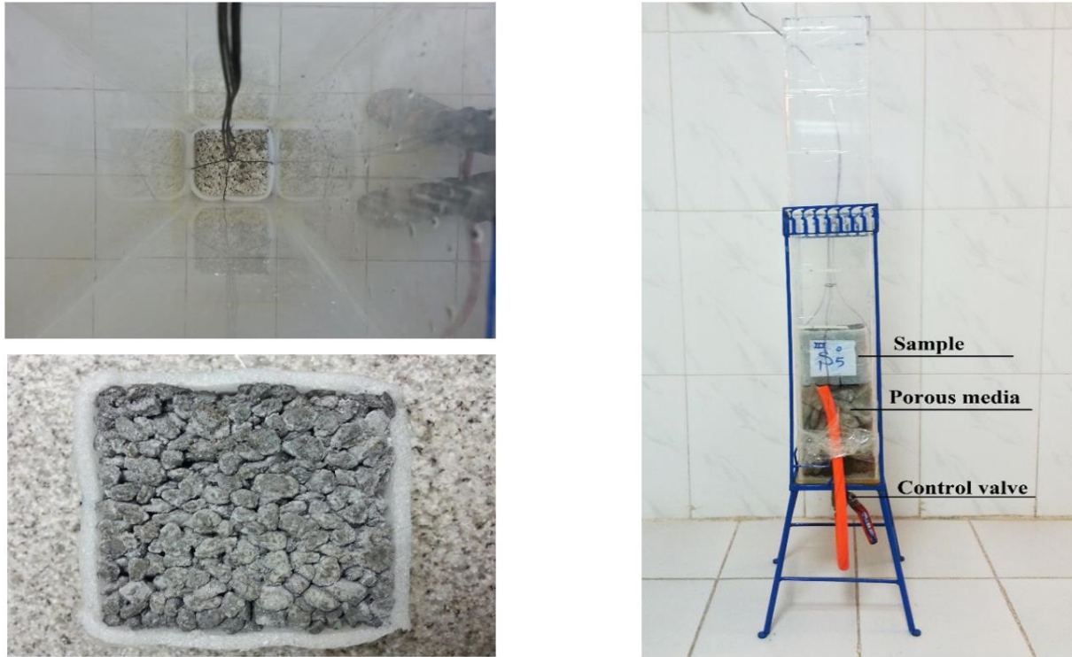
Fig. 2. Permeability measuring device.
