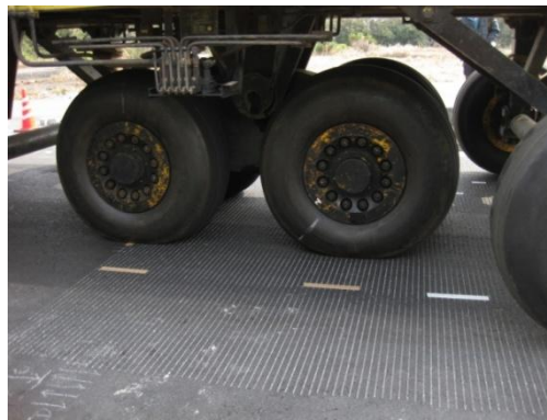
Fig. 7. Full-scale wheel loading at the surface with grooving.
