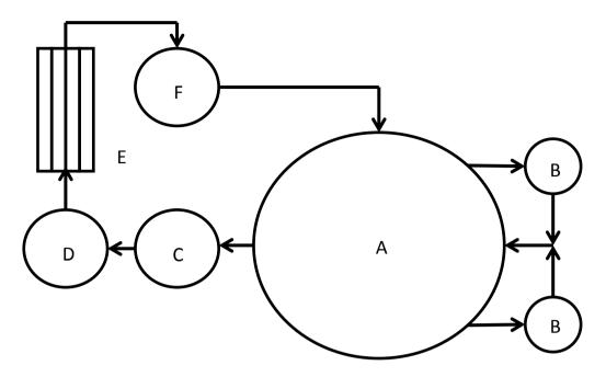
Fig. 1. Schematic diagram of the recirculating aquaculture system: (A) rearing tank (B) solids separating units (C) nitrifying biofilters unit (D) methanol addition and mixing unit (E) tubular denitrifying reactor and (F) aeration unit.
