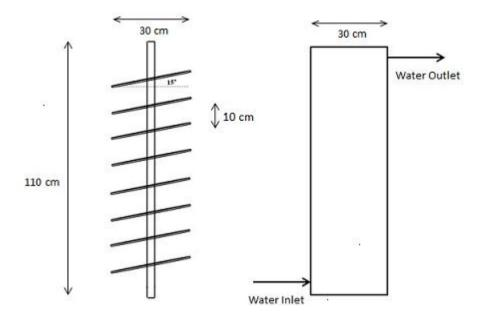
Fig. 2. Schematic diagram of the solids separating unit: (left) the interior design with 8-leveled discs (right) exterior sketch showing water inlet and outlet.
