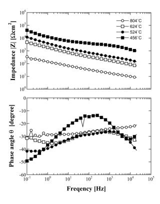
Fig. 9. Impedance behavior for aluminide diffusion coating on Inconel 600 and its change with temperature under molten sulfate film during the second thermal cycle. The test was conducted with two-electrode configuration electrochemical cell.
