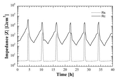
Fig. 10. Monitoring results for Inconel 600 during 6 thermal cycles under molten sulfate film with two-electrode configuration cell. R<sub>c</sub>: corrosion resistance, R<sub>s</sub>: solution resistance of molten sulfate film.
