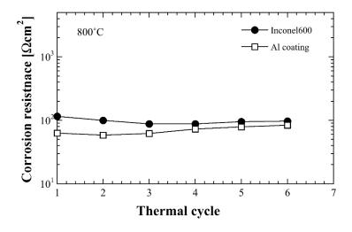
Fig. 7. Changes in corrosion resistance Rc at 800°C during 6 thermal cycles test for Inconel 600 and aluminide coating under molten sulfate film. The test was conducted with three-electrode configuration.
