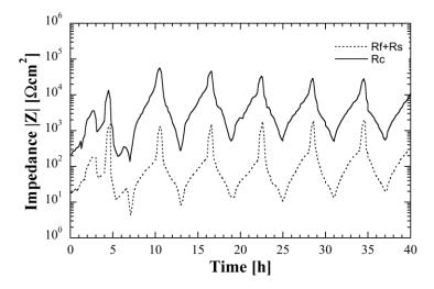
Fig. 11. Monitoring result for aluminide diffusion coating on Inconel 600 during 6 thermal cycles under molten sulfate film with two-electrode configuration cell. R<sub>c</sub>: corrosion resistance, R<sub>f</sub>: resistance of aluminum oxide layer, R<sub>s</sub>: solution resistance of molten sulfate film.
