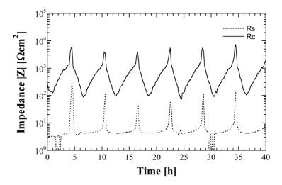
Fig. 13. Monitoring results for Inconel 600 during 6 thermal cycles under molten sulfate film with twoelectrode configuration cell. R<sub>c</sub>: corrosion resistance, R<sub>s</sub>: solution resistance of molten sulfate film.
