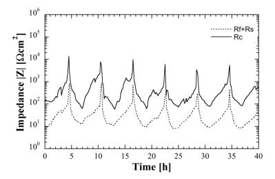
Fig. 6. Monitoring result for aluminide diffusion coating on Inconel 600 during 6 thermal cycles under molten sulfate film with three-electrode configuration cell. R<sub>c</sub>: corrosion resistance, R<sub>f</sub>: resistance of aluminum oxide layer, R<sub>s</sub>: solution resistance of molten sulfate film.
