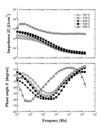
Fig. 3. Impedance behavior for Inconel 600 and its change with temperature under molten sulfate film during the second thermal cycle. The test was conducted with three-electrode configuration electrochemical cell.
