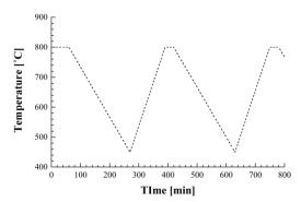
Fig. 1. Schematic diagram of thermal cycle. Temperature range: 450°C~800°C, raising rate: 3°C/min, lowering rate: 1.6°C/min, holding time at 800°C: 30min (60 min for the first cycle).
