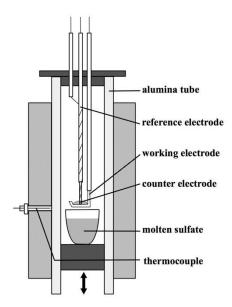
Fig. 2. Electrochemical cell designed for electrochemical measurements under molten salt film condition.
