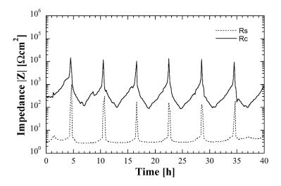
Fig. 5. Monitoring results for Inconel 600 during 6 thermal cycles under molten sulfate film with three-electrode configuration cell. R<sub>c</sub>: corrosion resistance, R<sub>s</sub>: solution resistance of molten sulfate film.
