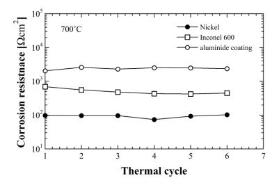
Fig. 14. Changes in corrosion resistance Rc at 700°C during 6 thermal cycles test for nickel, Inconel 600 and aluminide coating under molten sulfate film. The test was conducted with two-electrode configuration.
