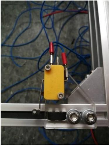
Fig. 8. Installation of limiting switch.
