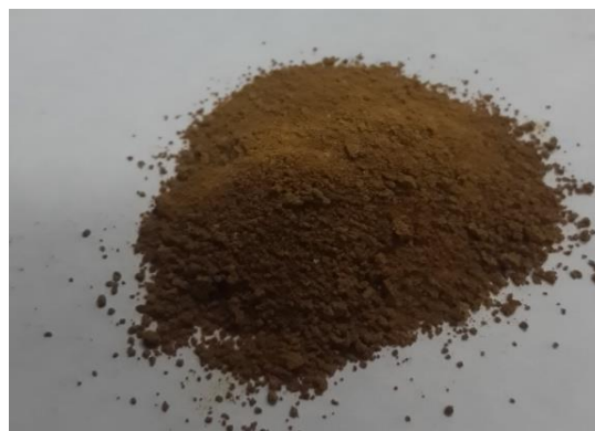
Fig. 7. Lanthanide hydroxide from precipitation reaction with sodium phosphate salt.
