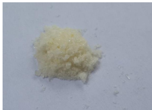
Fig. 6. Lanthanide hydroxide ( \text{Ln}(\text{OH})_3 ) produced from sodium sulfate precipitation process.
