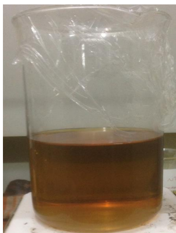
Fig. 5. Leachate solution of Indonesian low grade bauxite from solid-liquid extraction.
