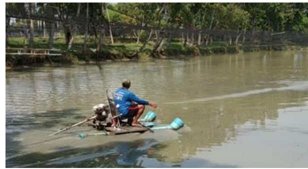
(a) The boat dragging rake and chains
