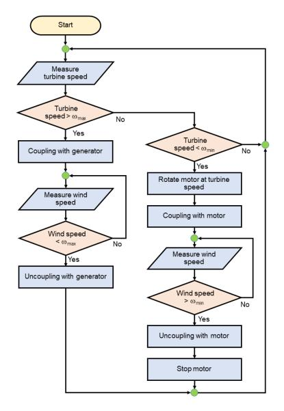
Fig. 8. The flowchart of the proposed control algorithm.
