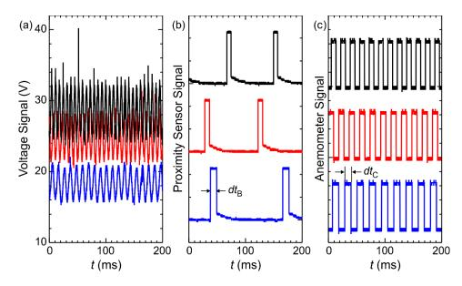
Fig. 6. The recorded signals at three different wind speeds: (a) voltage signal at the generator terminal, (b) proximity sensor signal and (c) anemometer signal.
