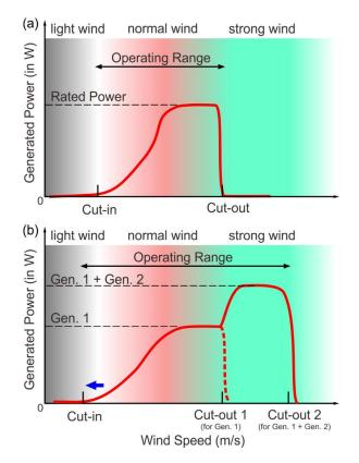
Fig. 1. Schematics of generated power vs. wind speed in (a) a conventional wind turbine and (b) the proposed hybrid wind turbine.
