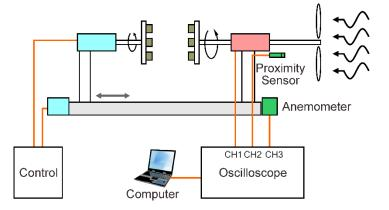
Fig. 5. Schematic diagram of the setup for testing experiment.
