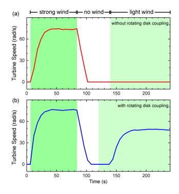
Fig. 7. The recorded turbine speeds in case that the rotating PM disk is (a) unused and (b) coupled when the wind speed is low.
