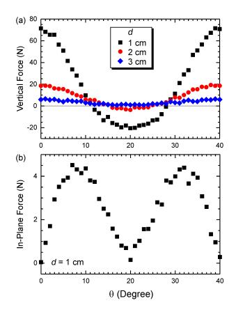
Fig. 3. (a) Calculated vertical pushing force between the disks when the distance *d* is 1, 2, and 3 cm. (b) Calculated in-plane pushing force between the disk when d = 1 cm. Zero in-plane force is observed at  $\theta = 0^{\circ}$  and  $20^{\circ}$ .
