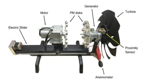
Fig. 4. Photo of prototype of the developed hybrid wind turbine. It consists of a pair of coupling PM disks, motor, electric slider, generator, turbine, proximity sensor and anemometer.
