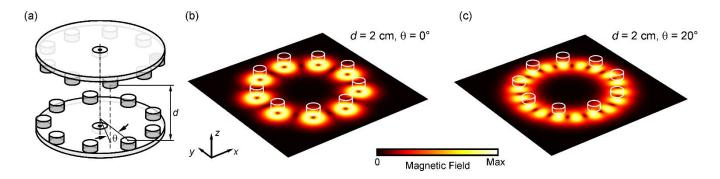
Fig. 2. (a) Schematic of the simulated coupling disks. Magnetic field distribution on the middle plane when between the disks when the magnets are (b) aligned and (c) interdigitated.
