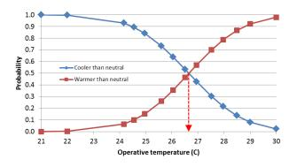
Fig. 4. Probit regression model fitted to thermal sensation percentages.
