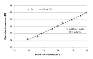
Fig. 2. The surveyed operative and room air temperatures.
