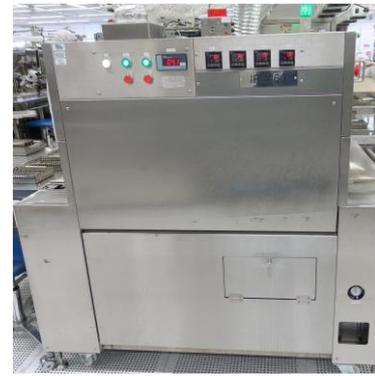
Fig. 4. IR oven for completely curing the adhesive joint.
