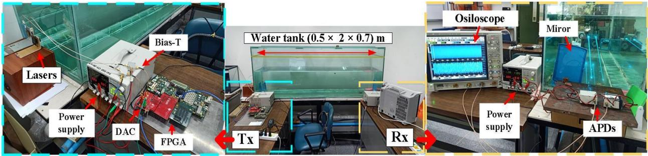
Fig. 2. Experimental setup of UOWC SC-FDM communication systems.
