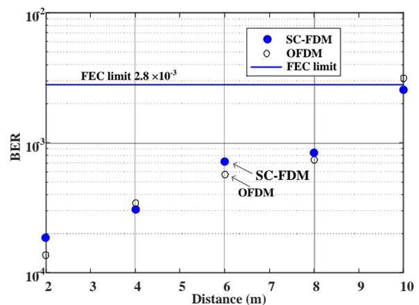
Fig. 3. BER performance comparison of SC-FDM and OFDM for 8-QAM.
