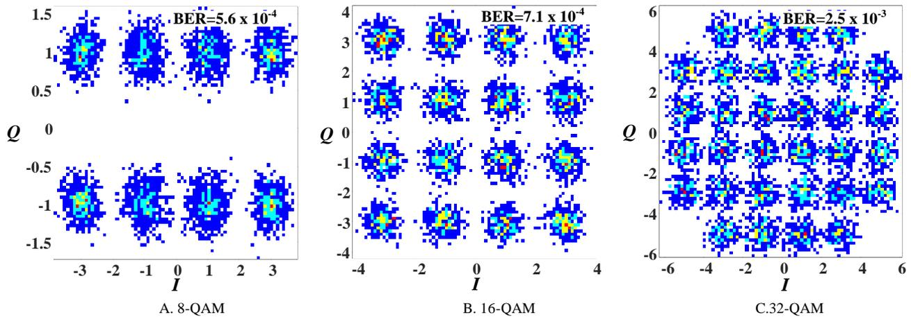
Fig. 4. Constellation plot at 6 m for: A. 8-QAM, B. 16-QAM, and C. 32-QAM for SC-FDM.
