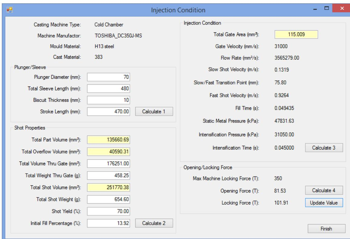
Fig. 11. A user interface for determination of injection condition.
