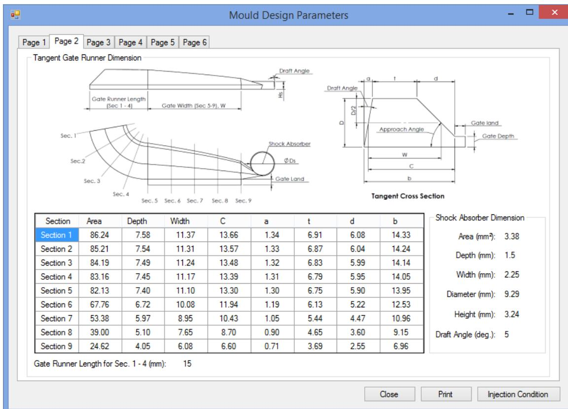
Fig. 10. A user interface for mold design parameters.
