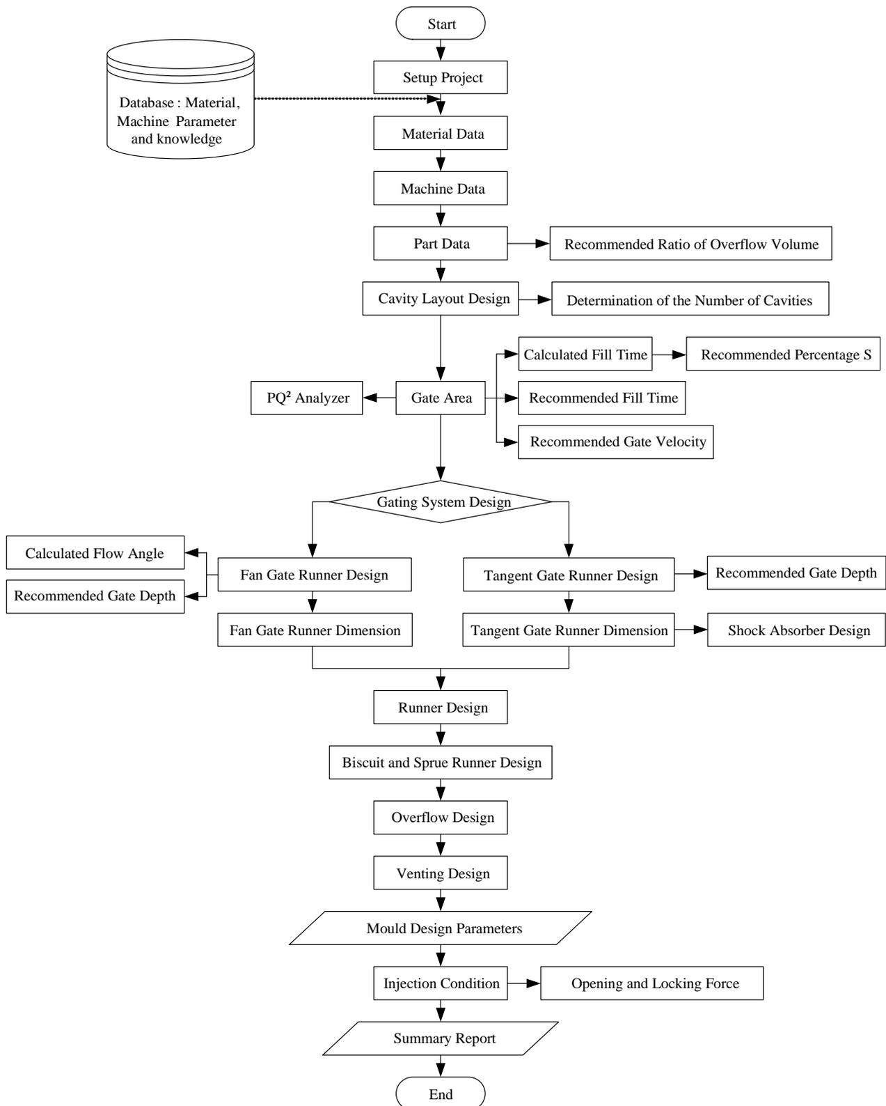
Fig. 13. Flowchart of computer aided program for aluminum die-casting mold design.
