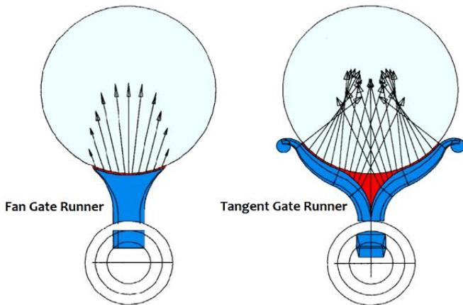
Fig. 2. Fan Gate runner and tangent gate structure [46].
