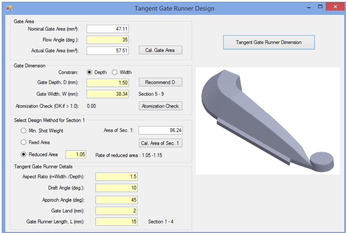
Fig. 9. A user interface for gate runner design.
