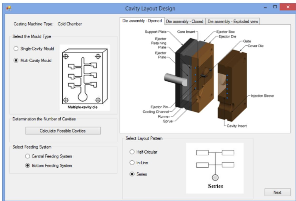
Fig. 7. A user interface for cavity layout design.
