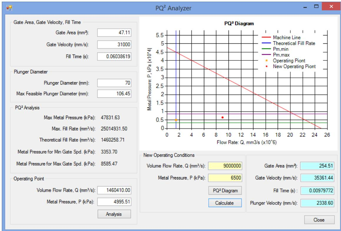
Fig. 8. A user interface for PQ<sup>2</sup> analyzer.
