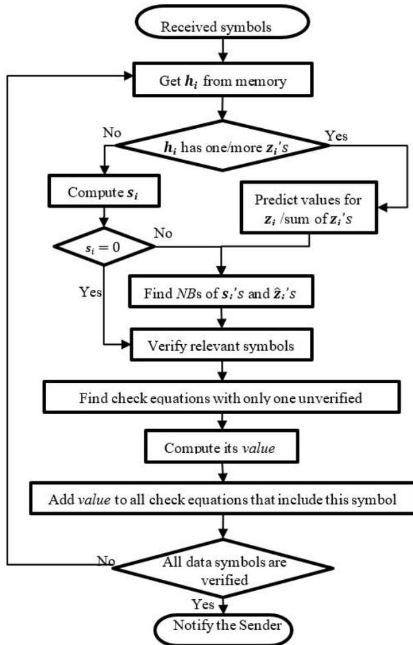
Fig. 2. Flowchart of the proposed decoding algorithm. Abbreviations: NB = null combination;  $h_i$  = check equation;  $z_i$  = erased symbol,  $z_i$  = predicted value.
