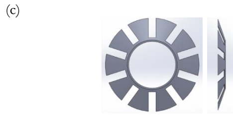
Fig. 2. Types of turbulator (a) Orbicular-ring turbulator (ORT), (b) Pyramidal-ring turbulator (PRT), (c) Cogwheel-ring turbulator (CRT) with N = 10 .
