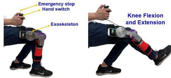
Fig. 9. Experimental setup for the active-assistive and resistive experiment.
