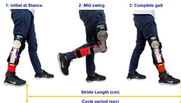
Fig. 17. Experimental setup and parameters employed in the computation for gait rehabilitation. The stride length and cycle period are determined using the length and time frame from the initial to the completion of gait.
