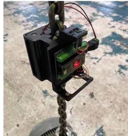
Fig. 6. Wireless sway angle measurement unit.
