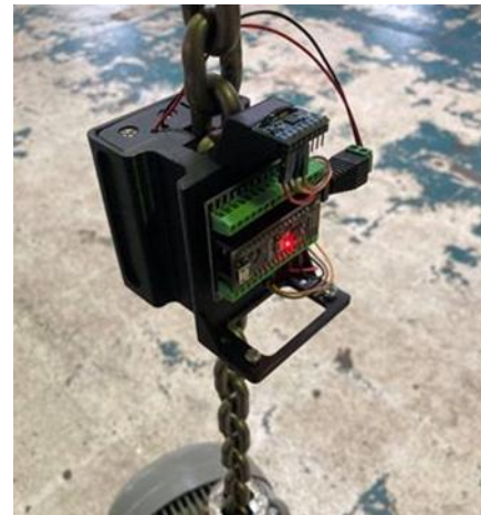
Fig. 6. Wireless sway angle measurement unit.
