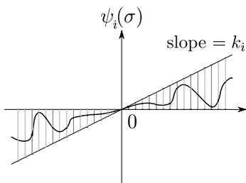
Fig. 3. Nonlinearity  $\psi_i \in \text{sector}[0, k_i]$ .
