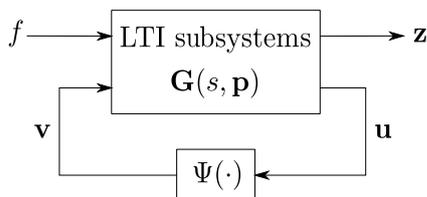
Fig. 1. General configuration for nonlinear control systems considered in the paper.
