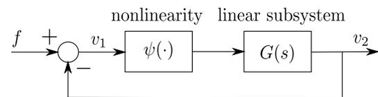
Fig. 2. Feedback control system with a nonlinearity.
