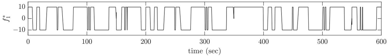
Fig. 6. Waveform of the test input  $f_1^*$  where  $\|f^*\|_\infty = 10$  and  $\|\dot{f}\|_\infty = 100$ .
