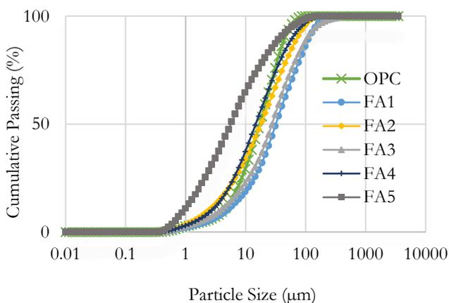
Fig. 2. Particle size distribution and mean particle size for OPC and FA.
