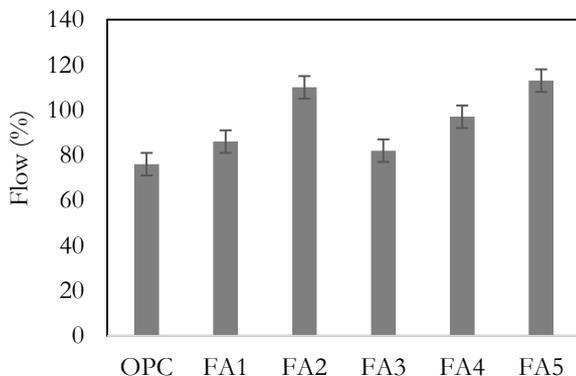
Fig. 3. Test results for flow of mortar.
