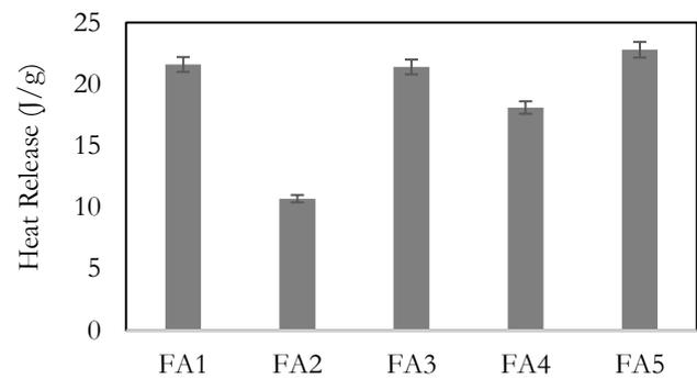
Fig. 7. Heat release after 10 days for FA at 40°C.
