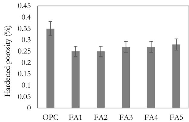
Fig. 4. Test results for hardened porosity.
