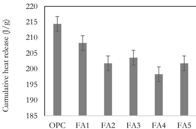
Fig. 6. Cumulative heat release after 7 days for blended FA-cement systems at 40°C.
