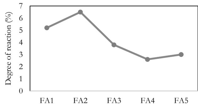
Fig. 8. Degree of reaction of FA at 40°C.
