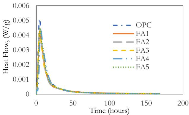
Fig. 5. Heat flow of blended FA-cement systems at 40°C.
