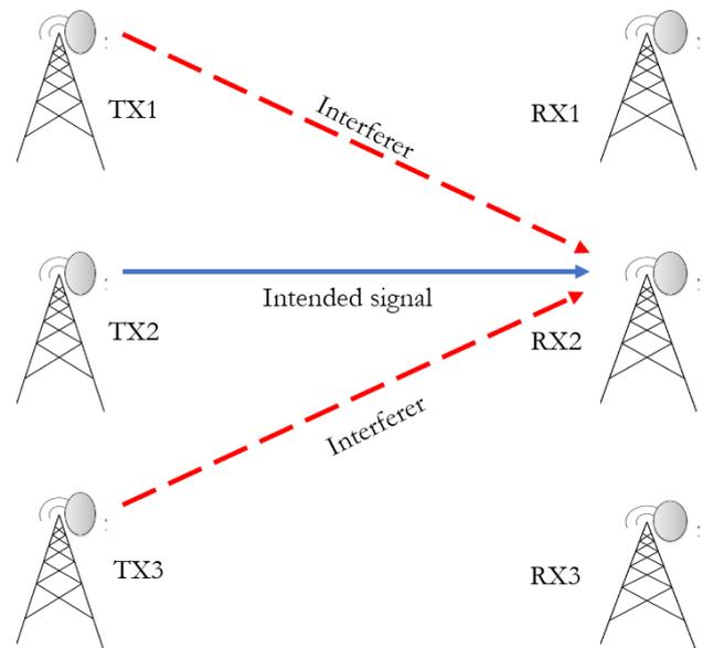
Fig. 2. SINR calculation model.
