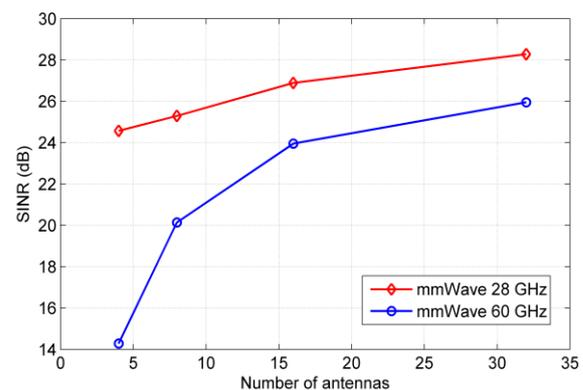
Fig. 8. SINR performance for mmWave MIMO 28 dan 60 GHz.
