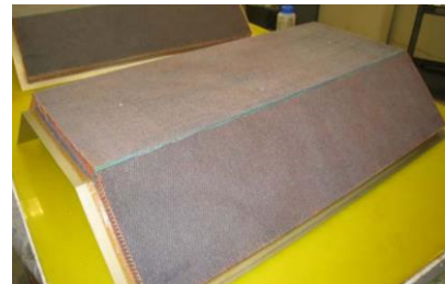
Fig. 12. Nomex honeycomb filling with Opaque Aerogel [43].
