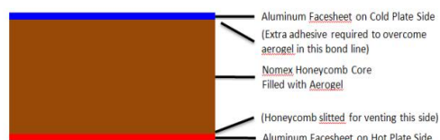
Fig. 11. Cross section of heat exchanger sandwich panel [43].
