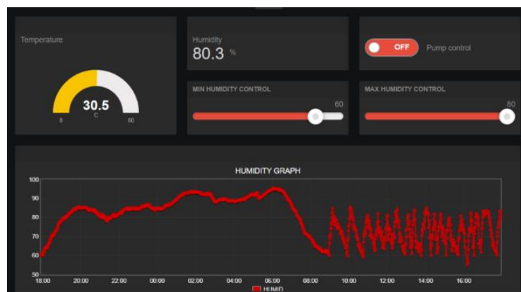
Fig. 5. The captured dashboard screen that shows the real-time data for temperature (upper left), humidity (upper center), water pump control (upper right), setpoints for the minimum/maximum humidity values (center slide bars) and time-series data of the humidity that is recorded for the last 24 hours (lower part).
