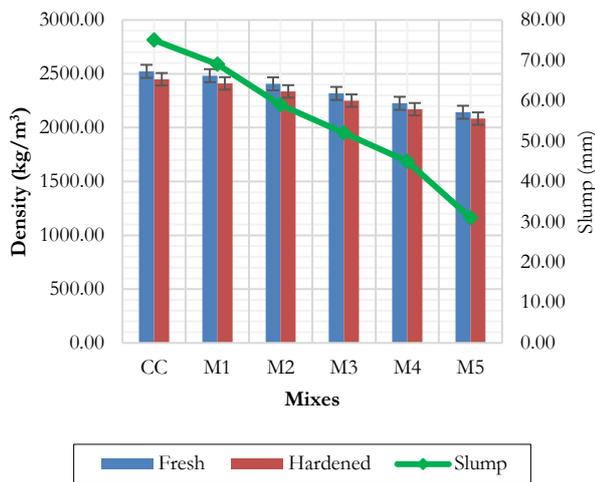
Fig. 2. Density and slump of FAC mixes.
