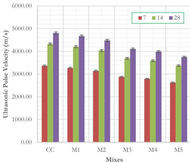
Fig. 5. Ultrasonic Pulse Velocity at various curing age.
