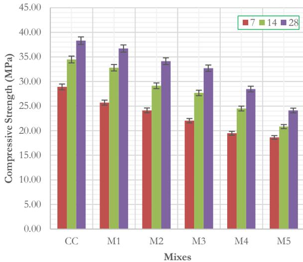
Fig. 4. Compressive strength at various curing age.
