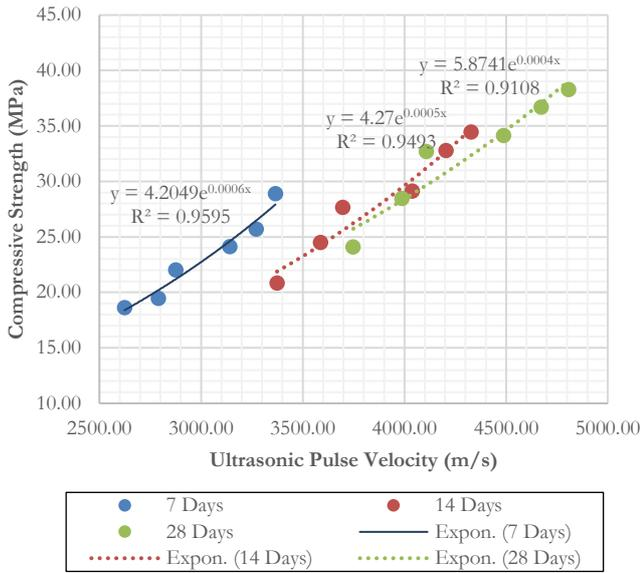
Fig. 7. Relationship between compressive strength and UPV in FAC on different curing ages.
