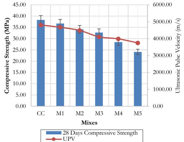
Fig. 3. UPV and Compressive strength in concrete specimens with varying levels of FAC replacement.
