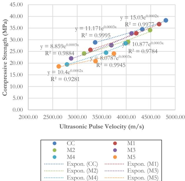
Fig. 8. Relationship between compressive strength and UPV in FAC on different mixes.
