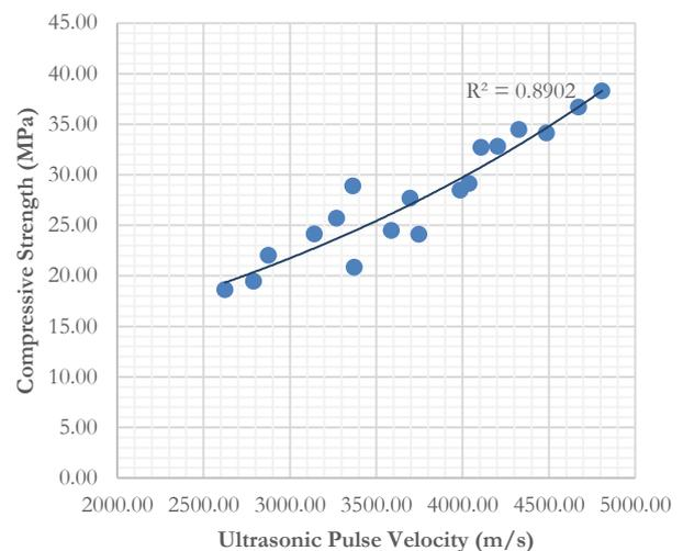
Fig. 6. Compressive Strength versus UPV.
