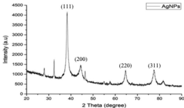
Fig. 9. XRD pattern analysis of P-jiringa-AgNPs.
