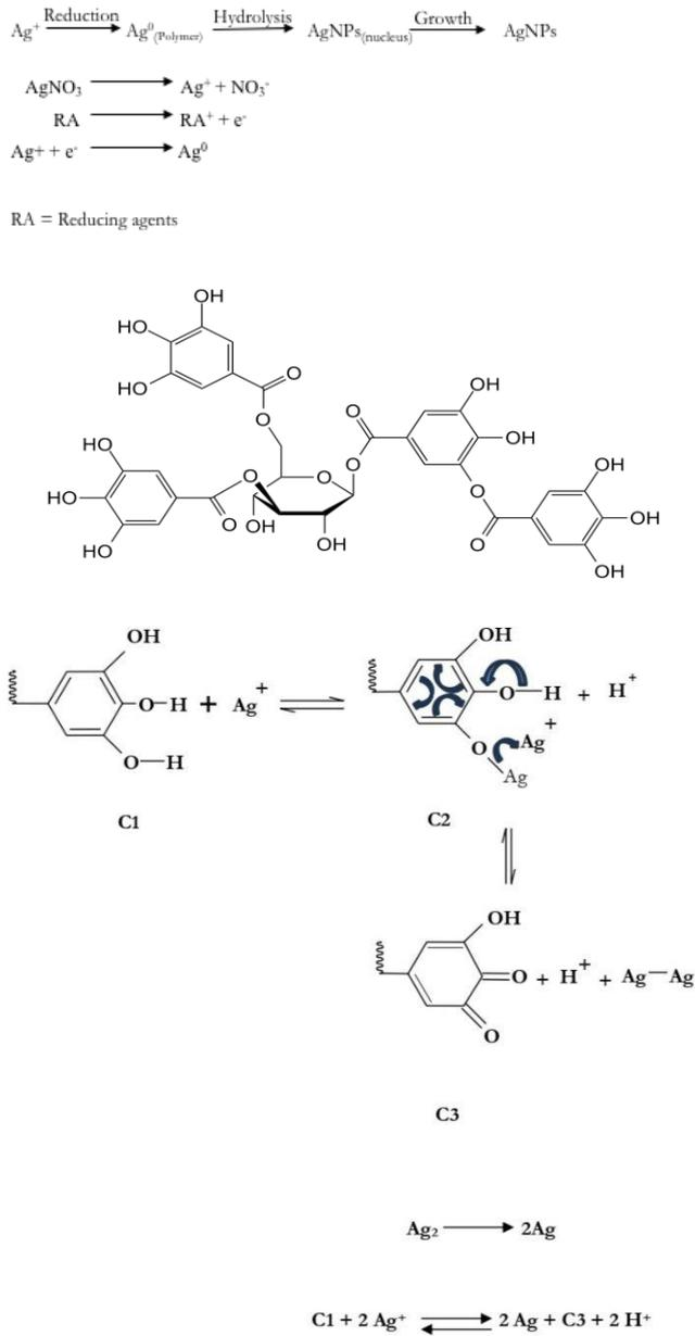
Fig. 5. Mechanism interaction between metal ions ( $Ag^+$ ) and reducing agents of tannin formation of AgNPs.
