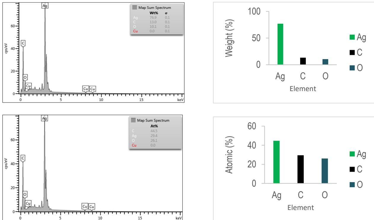
Fig. 8. Qualitative analysis of EDX elements (a) weight; (b) empirical atomic.
