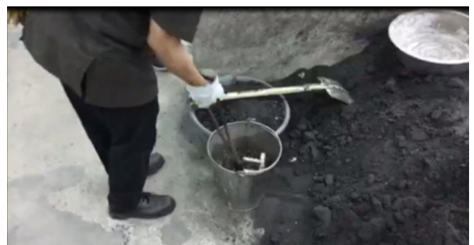
Fig. 48. Quenching step to rapidly cool down the workpiece.
