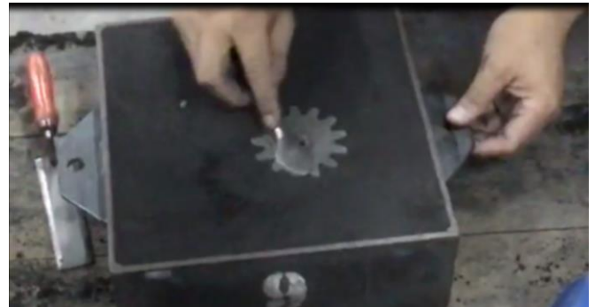
Fig. 46. Sand polishing step around the mold workpiece.
