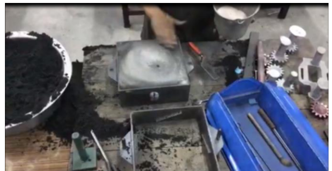
Fig. 47. Applying parting powder step to prevent the molding sand from sticking to the pattern or the mold box.
