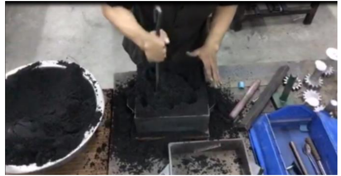
Fig. 45. Sand ramming step which improves mold strength and makes it dimensionally stable.
