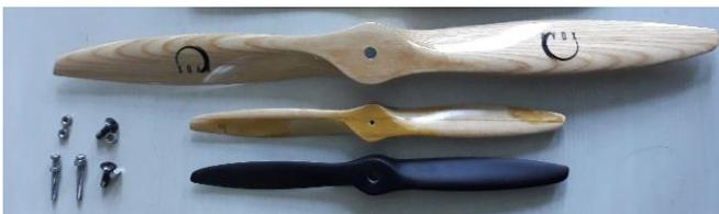
Fig. 3. Comparison between the original 18x10-inch propeller and the 1:0.555 scale carbon fiber propeller 10x6-inch model.
