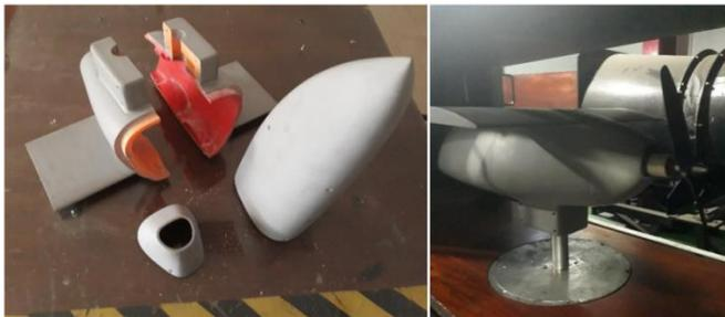
Fig. 10. Model of the experimental PUNA Alap-Alap BPPT fuselage with a scale factor of 1:0.555 and experimental setup.
