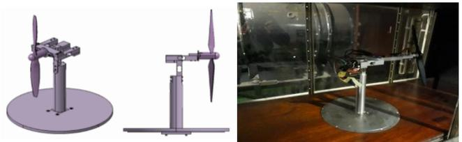
Fig.5. Experimental setup configuration for testing without fuselage.
