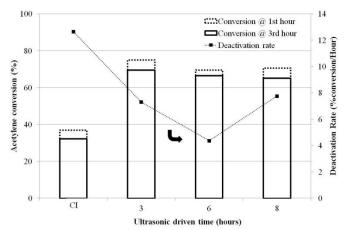
Fig. 3. %Acetylene conversion of samples prepared by using various ultrasonic driven times and comparing with CI sample (T = 180°C, ambient pressure and HCl/C<sub>2</sub>H<sub>2</sub> ratio = 1.1).
