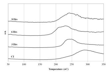
Fig. 2. H<sub>2</sub>-TPR profiles of gold catalysts synthesized by ultrasonic-assisted technique.
