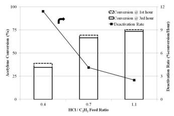
Fig. 5. Effect of  $HCl/C_2H_2$  feed ratio on % acetylene conversion and % VCM selectivity at steady state  $(T = 180^{\circ}C)$  and ambient pressure).
