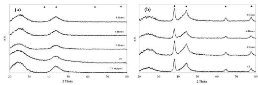
Fig. 1. X-Ray Diffraction (XRD) spectra of different driven time ultrasonic-assisted samples compared with pure carbon support (CK support) and conventional impregnation (CI). The fresh and used catalysts XRD spectra are shown in figure (a) and (b), respectively. (The triangle represents the Au<sup>0</sup> XRD peak position) [25]
