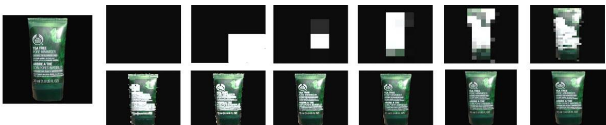
Fig. 10. On the left side is 4096x4096( 2^{12} \times 2^{12} ) pixels of input cosmetic Image. On the right side are images from different hierarchy of image pyramid.
