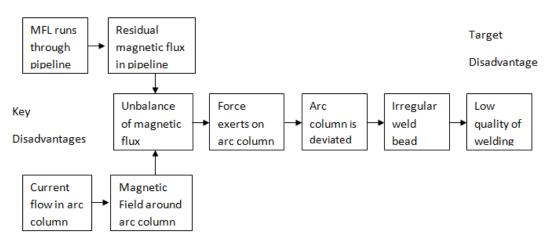
Fig. 5. Cause-Effect Chains Diagram of the problem of low quality of welding.
