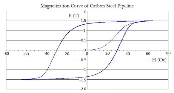
Fig. 20. Magnetic property of the carbon steel pipeline (API grades).
