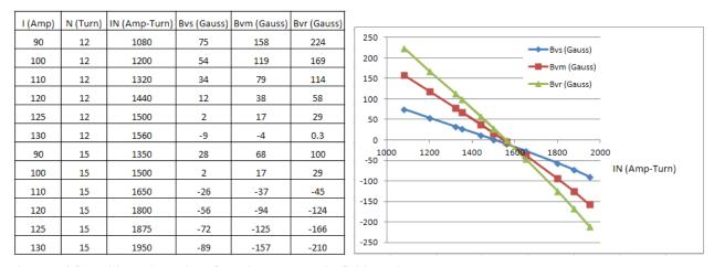
Fig. 24. The table and graphs of resultant magnetic fields at the V-groove.
