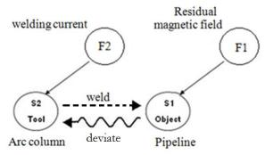
Fig. 9. Substance-field modeling and analysis.
