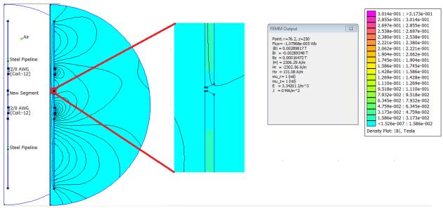
Fig. 22. Magnetic field simulation with compensation.
