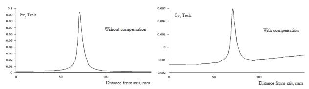
Fig. 23. Magnetic field variation at the V-groove from the axis inside the pipe to outside space.
