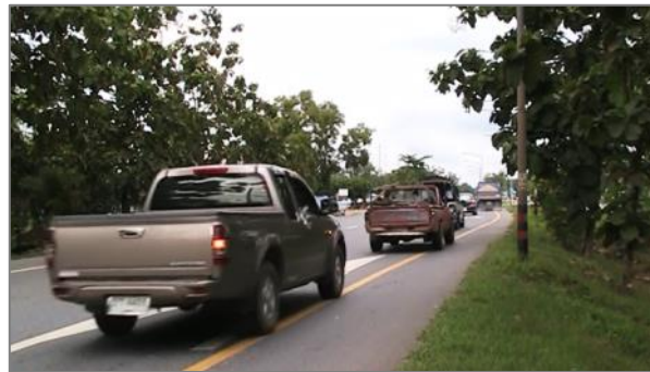
Fig. 3. Spillback effect by the queue of U-turing vehicles.
