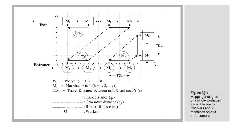
The U-line layouts illustrated in Table 2 are configured with symmetrical and rectangular shapes at the side ratios of 1/3 (1:1:1) and 1/9 (1:4:4), respectively. They are representative enough for the workable single U-line. The line consists of M
